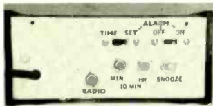
REAR VIEW, ALTAJ 4-DIGIT. Radio switch powers external radio for 45 minutes.
