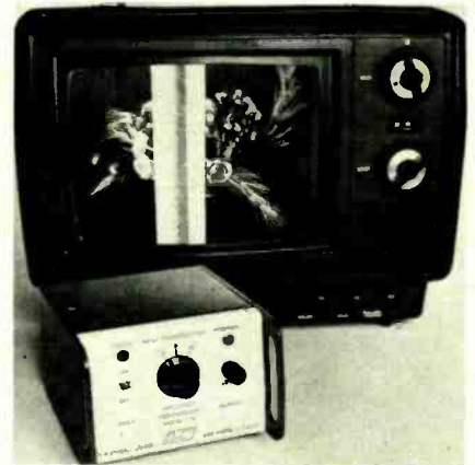
FIG. 7—DYNATRON MODEL 175 frequency comparator displays color-bar on the screen of an ordinary receiver.
