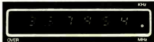
MHz display of 3.579548 MHz input (AUTO mode)
