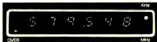
KHz display of overflow of 3.579548 MHz input (1SEC mode)
