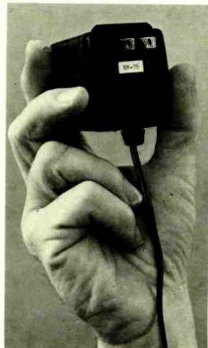
POWER comes from an external transformer.
