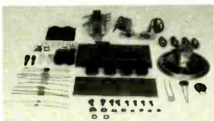
ALTAJ 4-DIGIT ALARM CLOCK parts layout. Includes a case, not shown.
