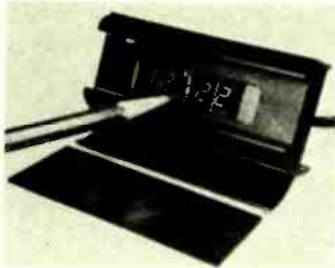
TWO MV-50 LED's between hour and minute displays form a pulsating colon that reads seconds in Space Age clock.
