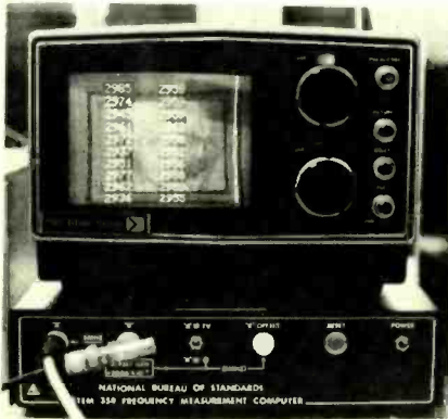
FIG. 4—PHASE COMPARISON permits calibration of oscillator to network color sub-carrier.
